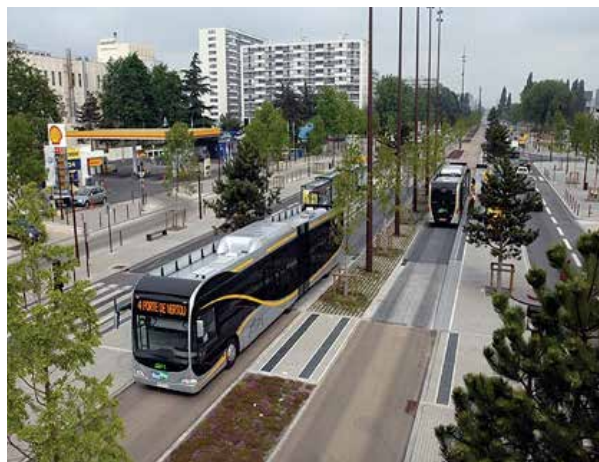
Figure 6 Typical configuration for median running
