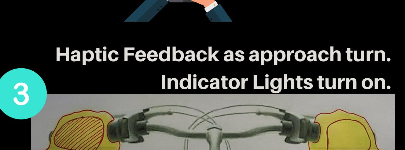
**Indicator Lights** on palm and back of hand on until turn completed.
