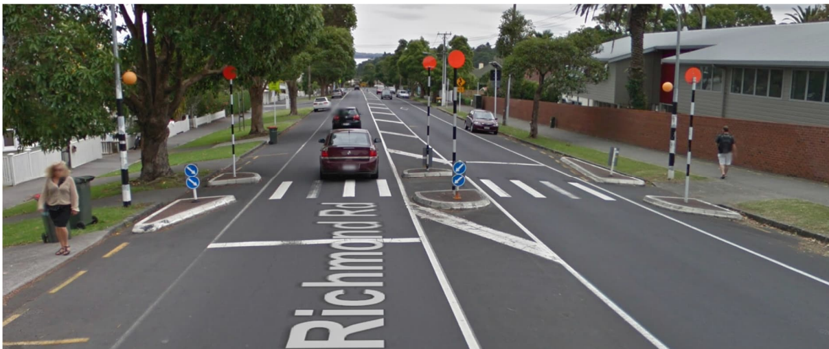
Figure 3.19: Crossing with flashing beacons and belisha beacon disks, Auckland (Image: Google Street View)
