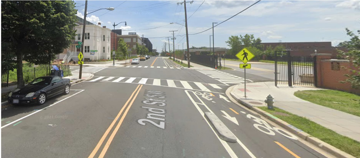
Figure 3.16: Zebra markings and warning signs at priority junction, Washington DC (Image: Google Street View)
