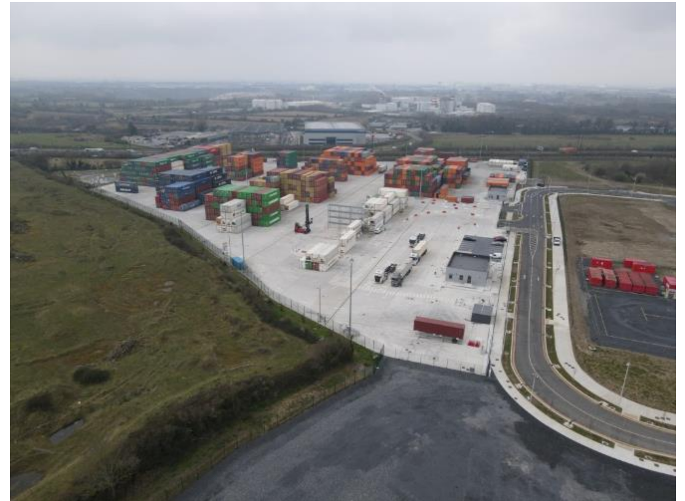
Figure 8 An Inland Port has been created to hold empty containers and free up space dockside (Dublin Port Company, 2022)
