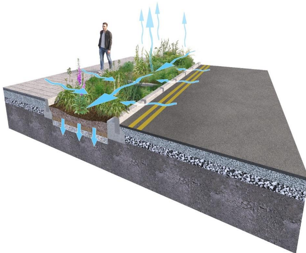
Figure 19 Illustration showing the principles of a Bioswale- needs to focus on differences from rain garden.
