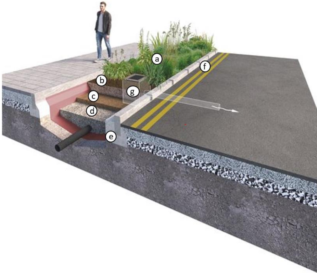
Figure 13 Illustration showing the components of a rain garden including underdrain and impermeable liner which should be provided where infiltration is not feasible.
