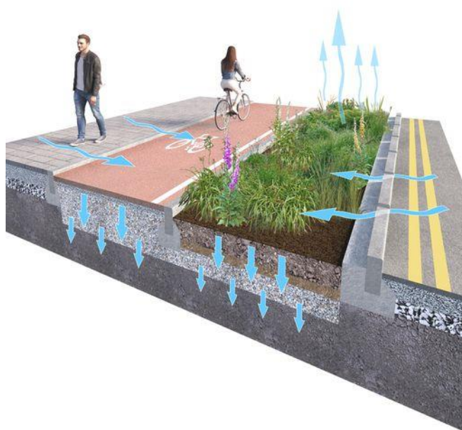
Figure 30 Permeable asphalt cycle path with raingarden
