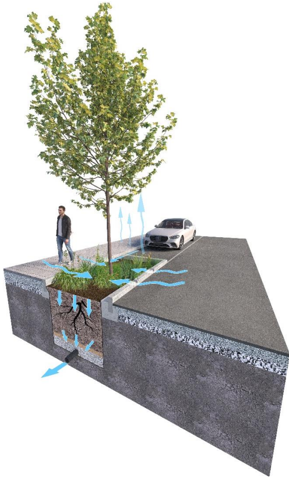
Figure 23 The principles of a SuDS tree pit
