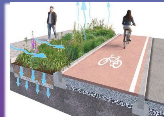
New cycle track on carriageway, existing verge repurposed (Could be incorporated as part of new CDM buffer requirements)
