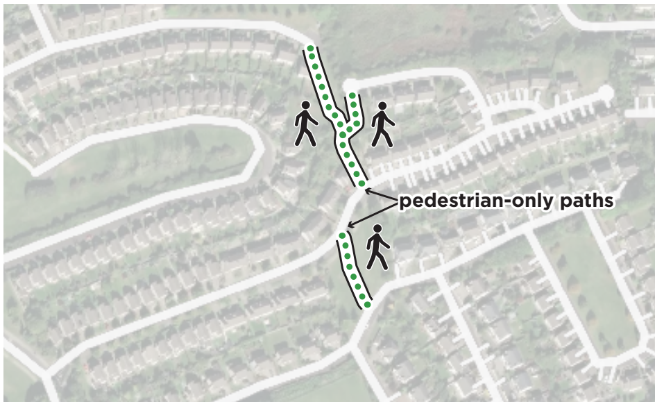
In this filtered permeability scheme, paths (shown as dotted green lines) shorten the walking and cycling routes to a park, the main street and bus stops.
