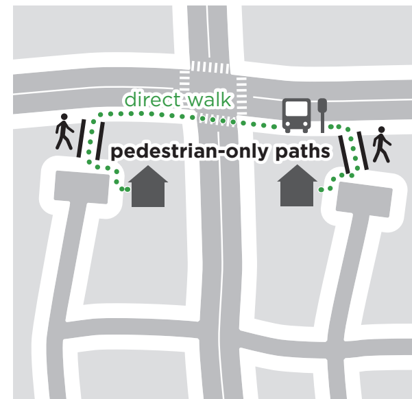
Cul-de-sacs without footpaths connecting them through (as on the left and at top) can make walks long and winding. Well-placed footpaths (as at bottom) shorten walking distances substantially.
