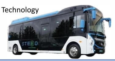
The Bus service will be carried out by an EV Higer bus, which is already in use on campus, the Higer bus has a range of 375km and only takes 2 hours to charge. The use of the EV bus will reduce emissions and increase the air quality in Galway City. Noise congestion will be reduced, providing a more comfortable journey for the passengers. The EV bus will have lower running costs and maintenance costs than a regular diesel bus.
