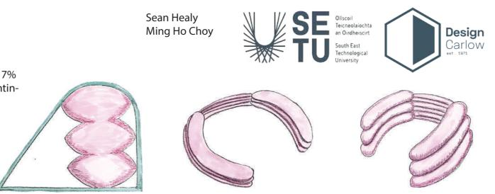
The inner cushion is a one-piece polymer construction which is crimped at the back during the blow-moulding process. This makes the cross-sectional area of these wall sections greater, and gives increased structural resistance, restricting inflation, and thereby preventing the uncomfortable effect of the neck being pushed away from the headrest by an inflated cushion.
