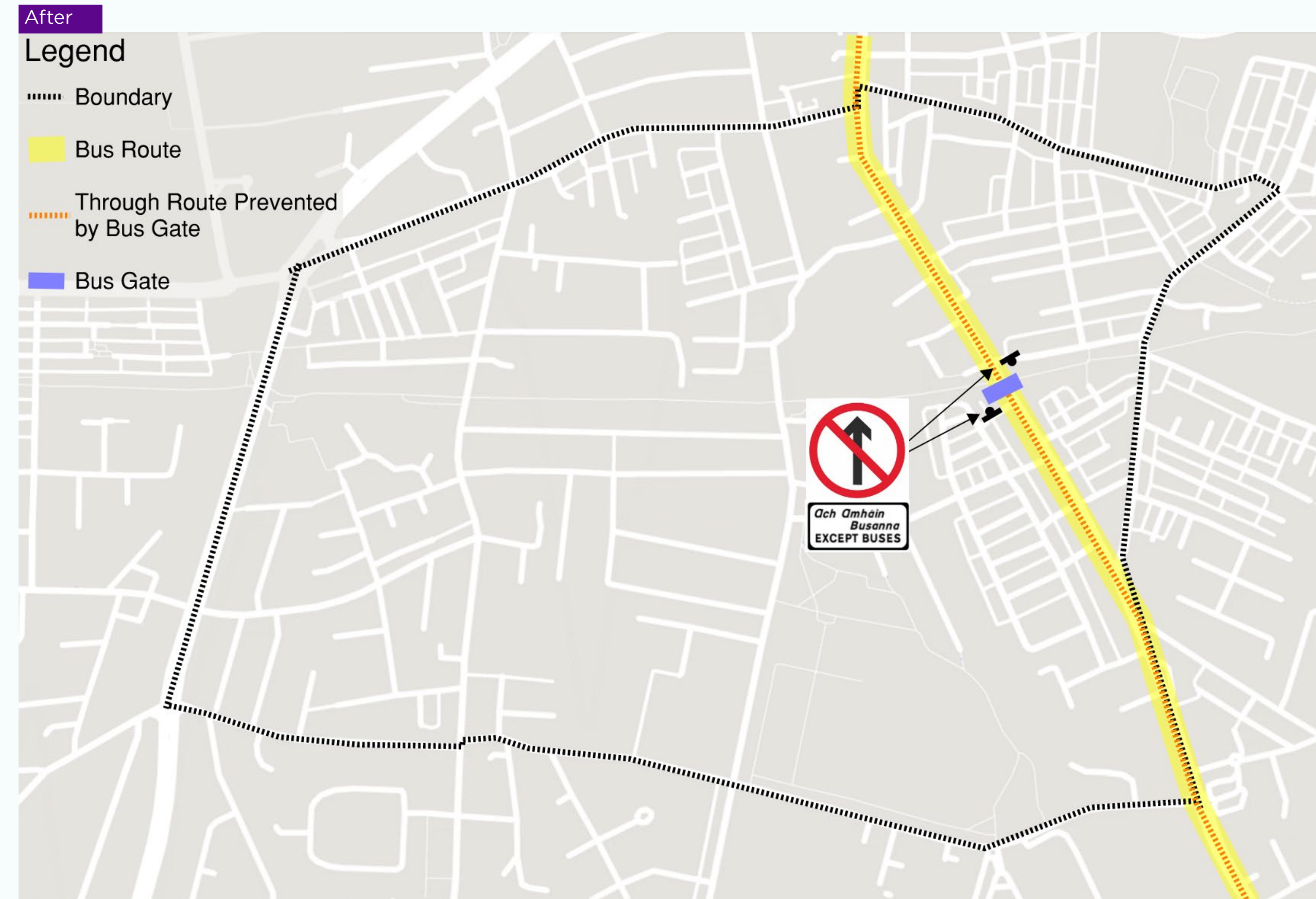
Figure 41: After: Bus gate provided to remove through route, local and boundary roads can serve as alternative routes for motor vehicles
