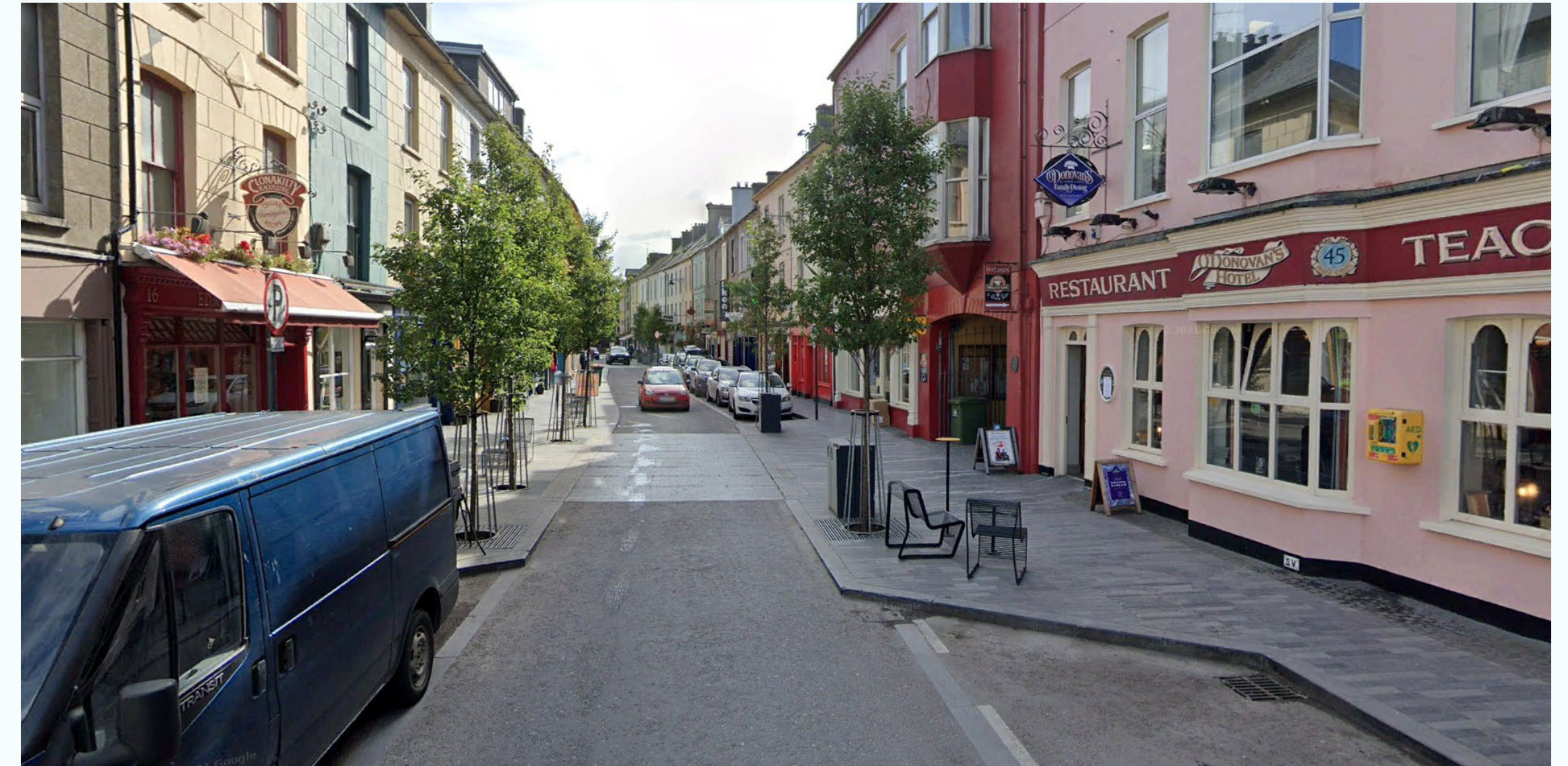
Figure 55: Mid-block build-out framing on-street parking bays and reducing pedestrian crossing distance, Clonakilty, Cork Source: © Google Street View 2019
