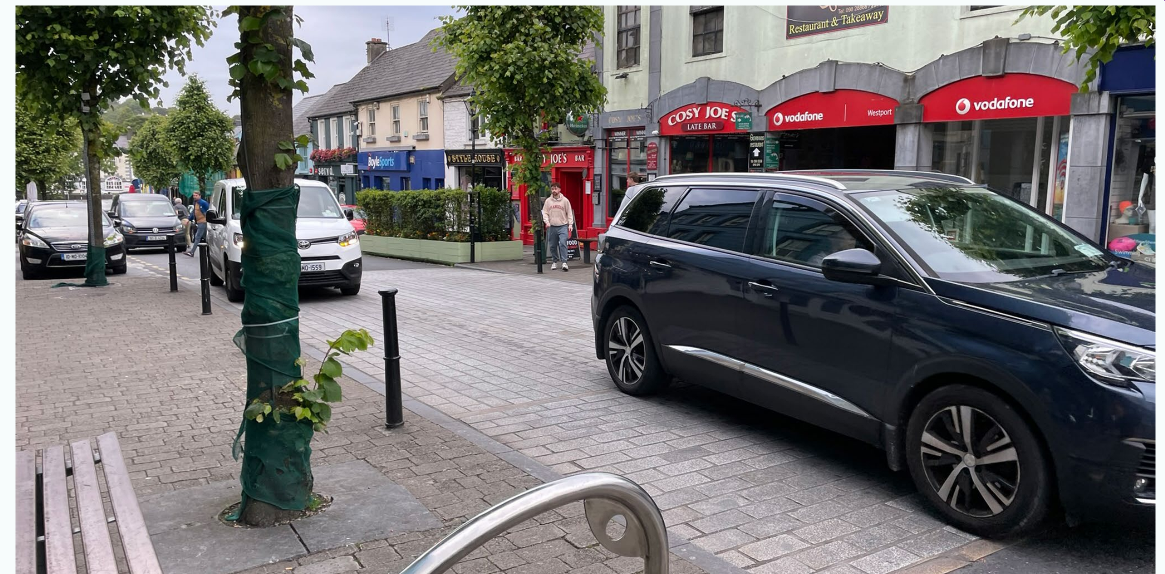
Figure 74: Raised table paired with unit pavers, Westport, Co. Mayo Link: © Google Street View 2023
