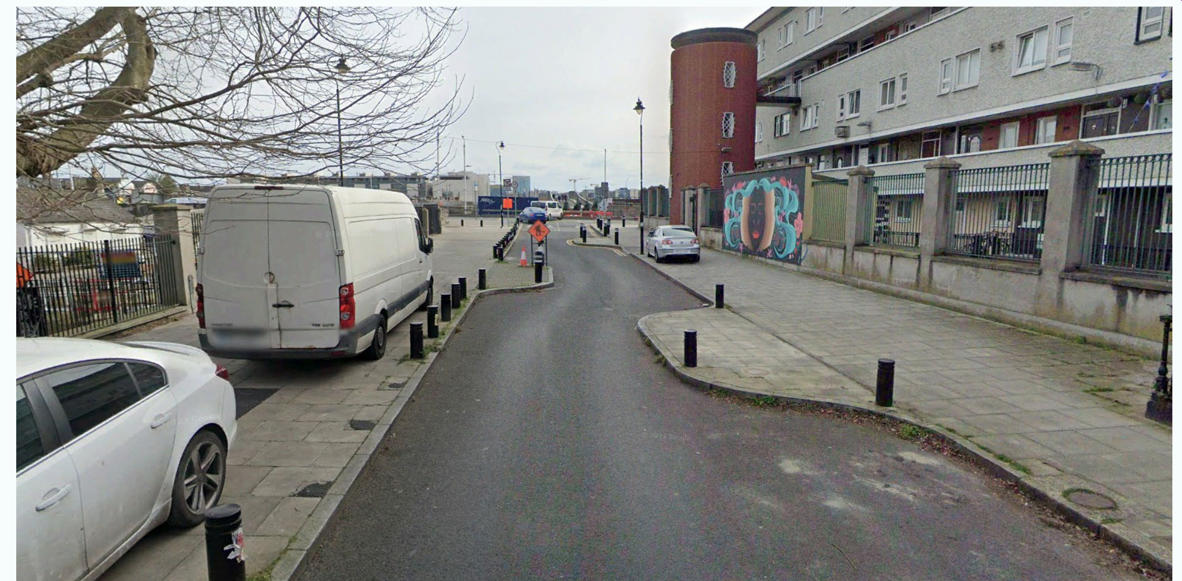
Figure 60: Chicane implemented with alternating build-outs, Dublin
