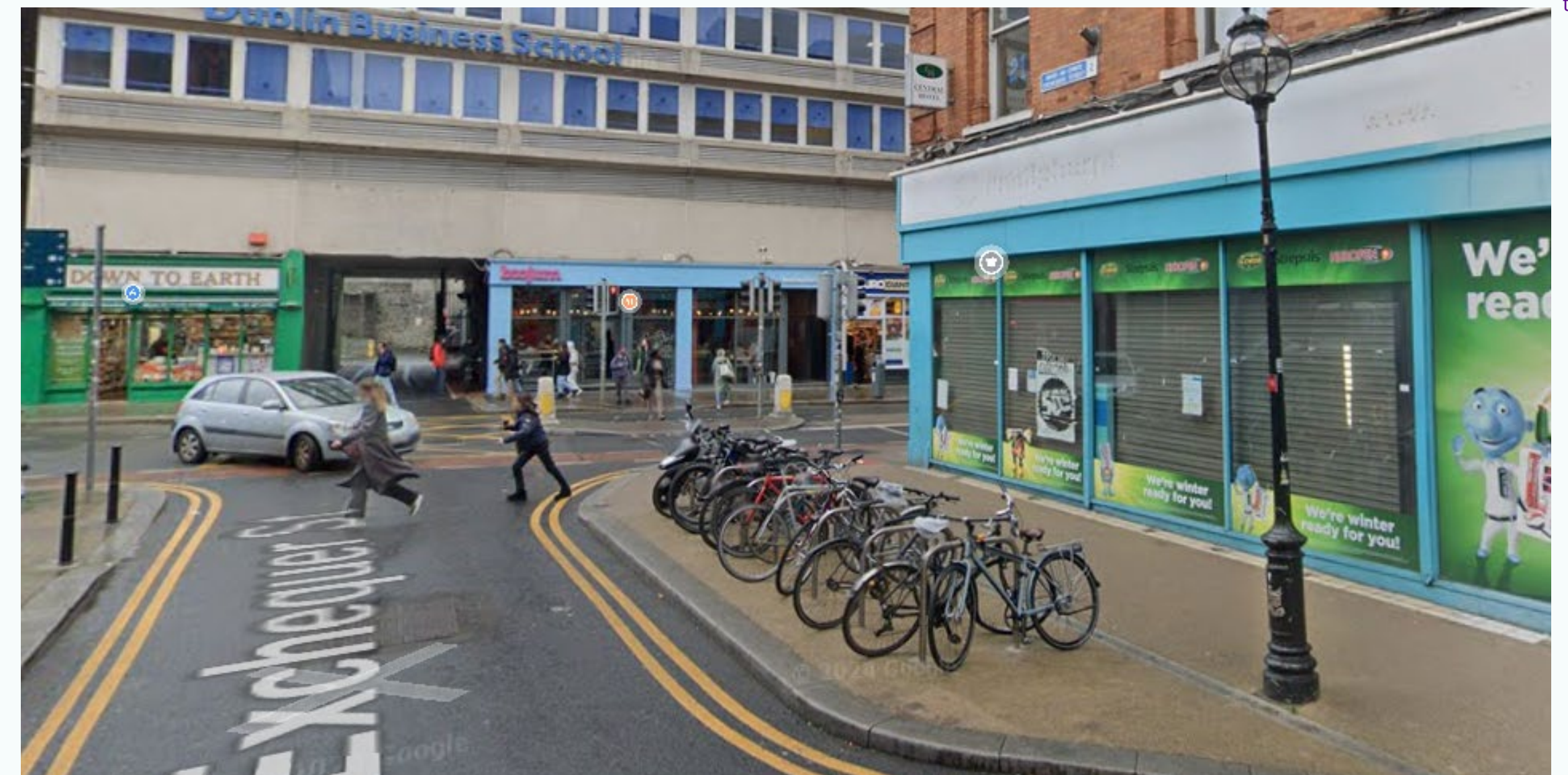
Figure 56: Build-out at a junction providing space for cycle parking, Dublin Source: © Google Street View 2022
