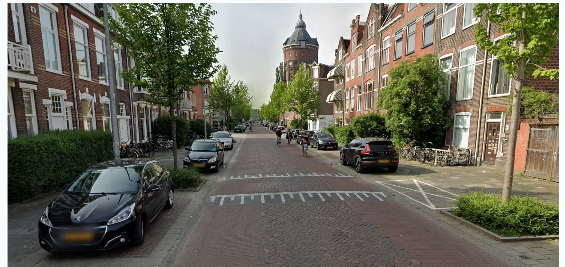
Figure 72: Cycle Street textured central strip and speed tables, Groningen, Netherlands Source: © Google Street View 2022
