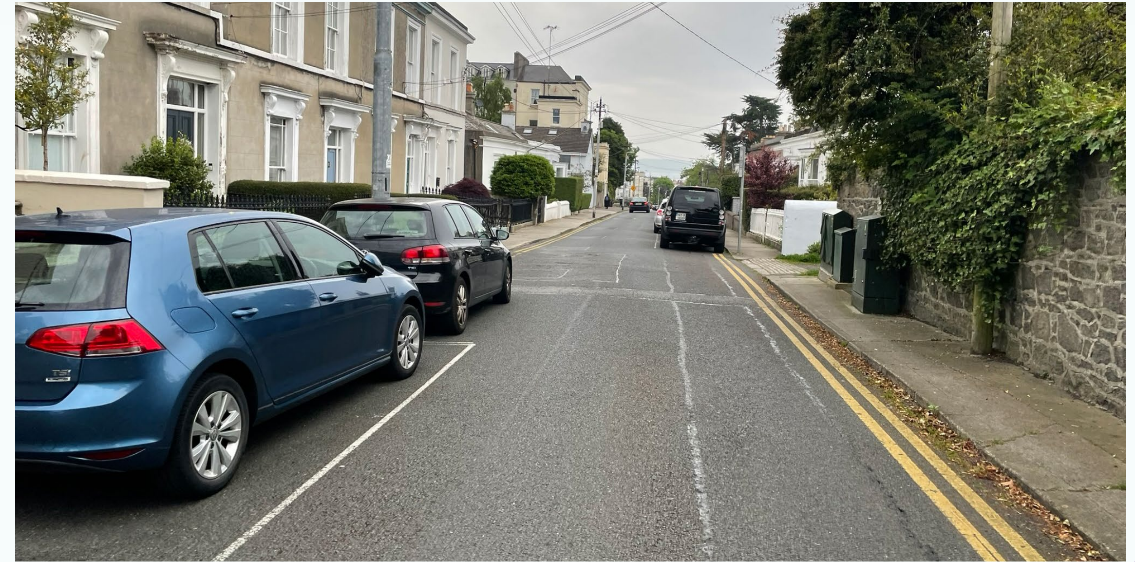
Figure 59: Alternating parking can create a chicane with minimal civil work, Dún Laoghaire
