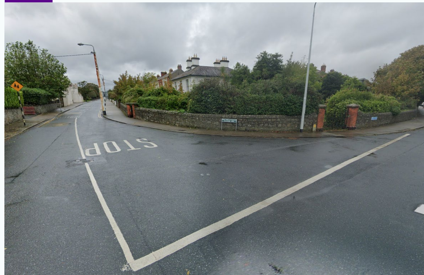
Figure 48: Corner radius reduction through reconstruction provided space for landscaping behind the footpath, Bullock, Co. Dublin Source: © Google Street View 2019 (Before), 2022 (After)
